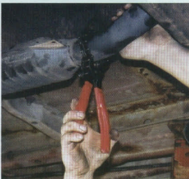
Weights were the NVH solution to the low-pitch groaning sounds from a mismatched exhaust system.
